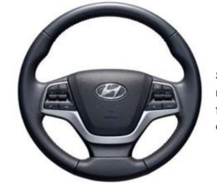
Steering wheel includes remote control functions for audio, cruise control and Bluetooth
