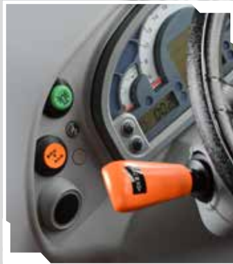
Hydraulic reverse shuttle with Stop&Go.
