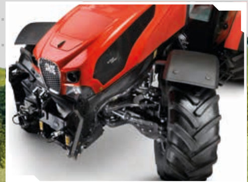
ActiveDrive independent front suspension.
