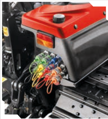
Up to 10-way rear hydraulic distributors.
