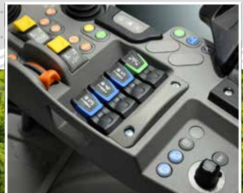
Electronically controlled hydraulic distributors.
