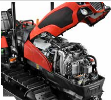
3 cylinder FARMotion engine.
