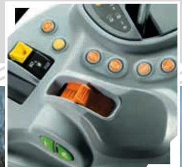
Electro-hydraulic controls for the main functions.
